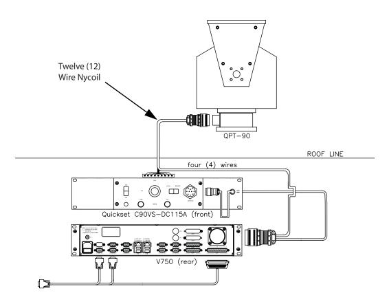
Figure 2–2. Typical Network Configuration
